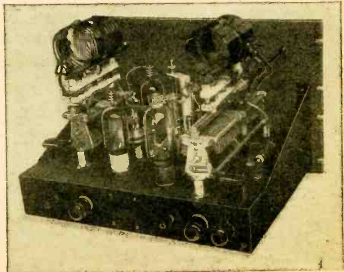
Front view of the dual r.f. power amplifier.
